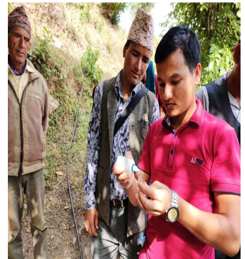
Mr. Badal Oli performing FRC test at Pilka WSS after chlorination
